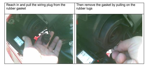
Now free the bulb/bulb holder unit Press in on the curly silver metal bit and then push it upwards to free it from the catch Rotate the catch to the side and lift the bulb/holder out
