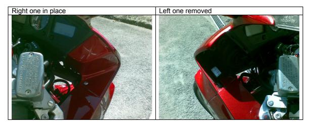
Getting this panel out without breaking anything is the most difficult task, so take your time. You will find access a lot easier if you put the bike on its centre stand, turn the steering towards the side you are working on, and protect the tank with a cloth, as you'll probably end up sticking bits on it.
