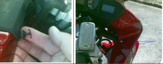
Once the fixings are out, free the outboard end of the panel and carefully free the panel from the various lugs/clips working towards the instrument panel.
